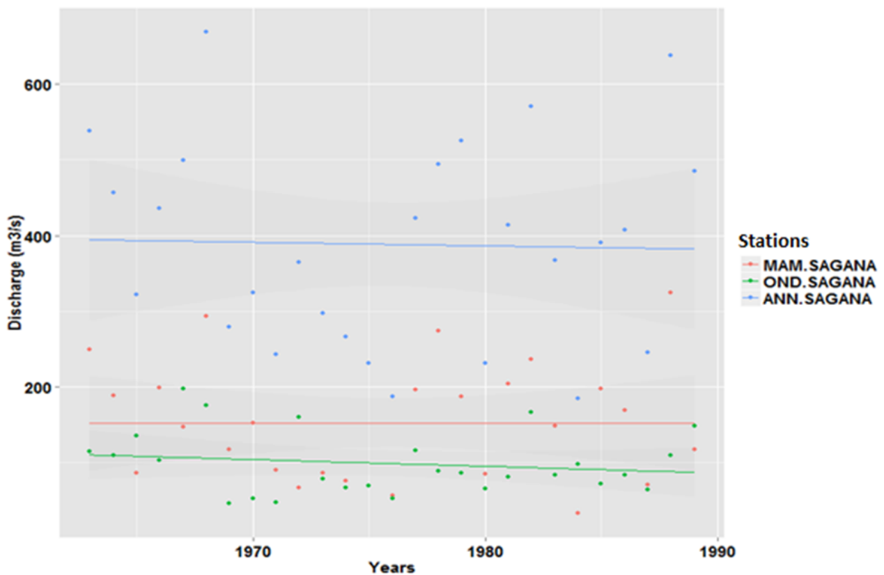
Figure 22: Trend analysis of the Discharge over the Sagana gauge station for the period 1963-1990
