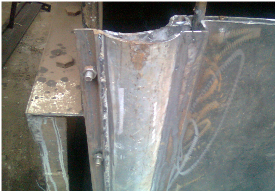
Fig 3.17: Detailed connection of upper and lower mould
