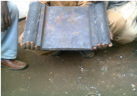
Fig 3.19: Output – Compressed plastic
