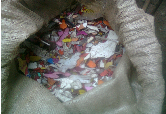
Fig 3.12: Recycled Plastic used to make substrate
