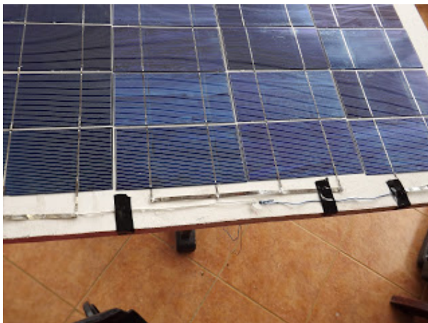
Fig: 3.8 Picture of Cells connected to bus wires
