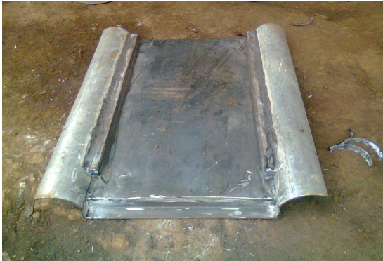
Fig 3.16: Reinforced upper mould
