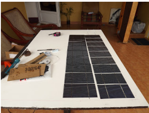
Fig 3.5: the cells connected in series
