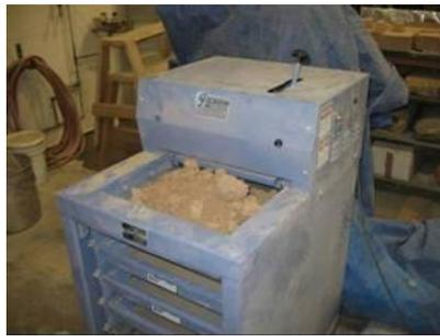
*Figure 8, Gilson Testing Screen Model TS-1*
