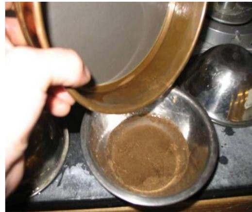
Figure 12 - #200 Sieve; Retained soil
