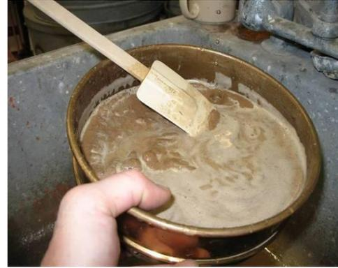
Figure 10 - #200 Sieve; mixing with water
