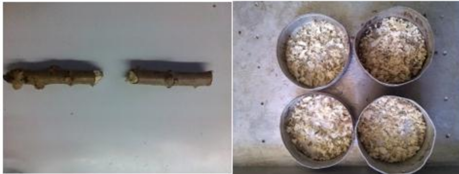
Plate 9: (a) cut cuttings for samples and (b) shredded sample in moisture dishes for moisture determination
