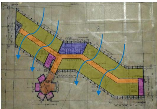
**Plate. 4.10: Plan of the tower showing cross ventilation. (Source: Architect author, 2016)**
