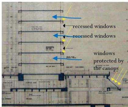
**Plate. 4.06: Section through the ICEA building showing air flow.** ←
