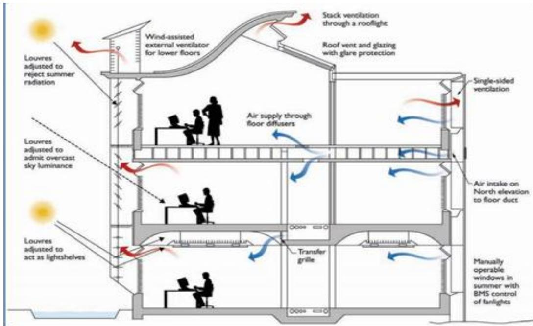
Plate. 2.02: A schematic showing the various natural ventilation strategies. (Source: [www.bsria.co.uk](http://www.bsria.co.uk), 2009)
