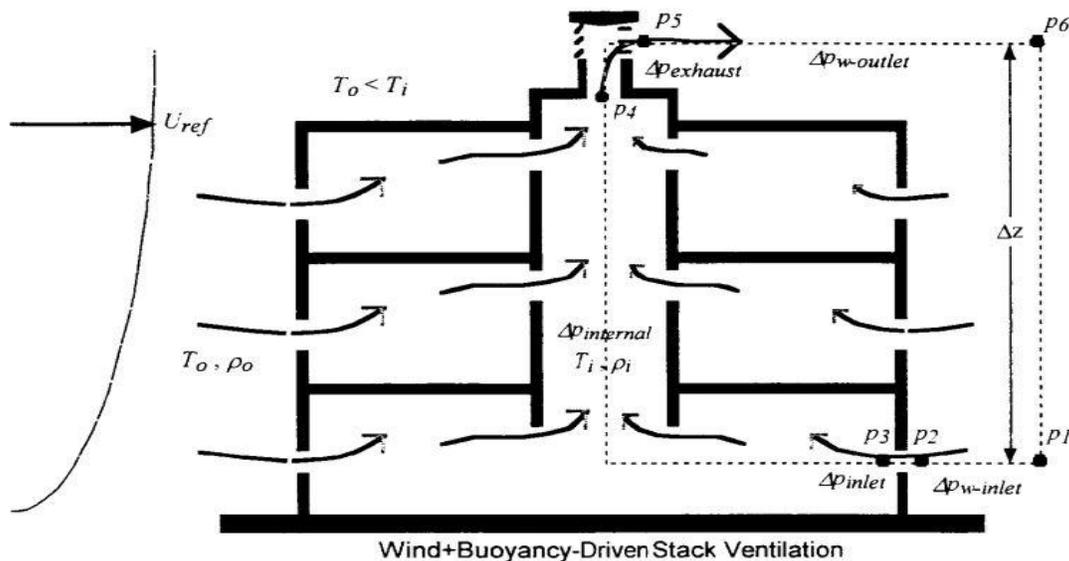
Plate. 2.01: Wind and buoyancy driven stack ventilation. (Source: Axley, 2001)
