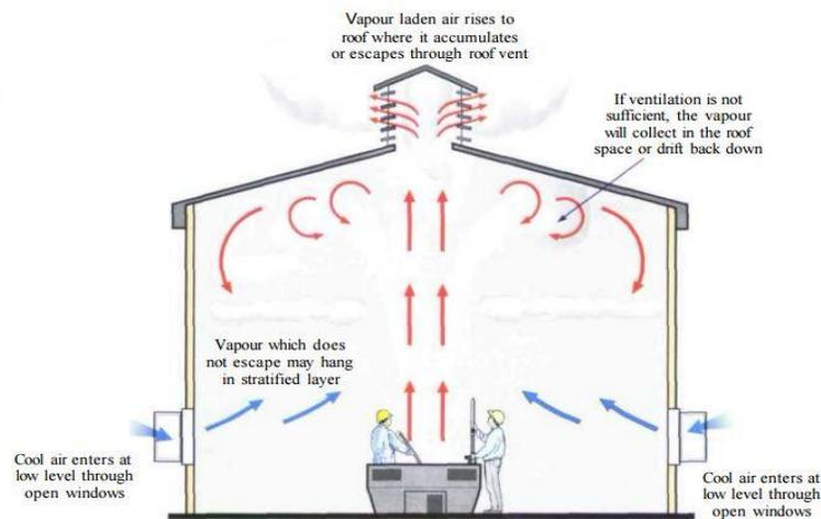
**Plate. 2.05: An example of stack ventilation to remove vapours through roof ventilators.**
