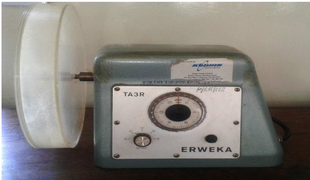
Plate 4: Friability testing machine
