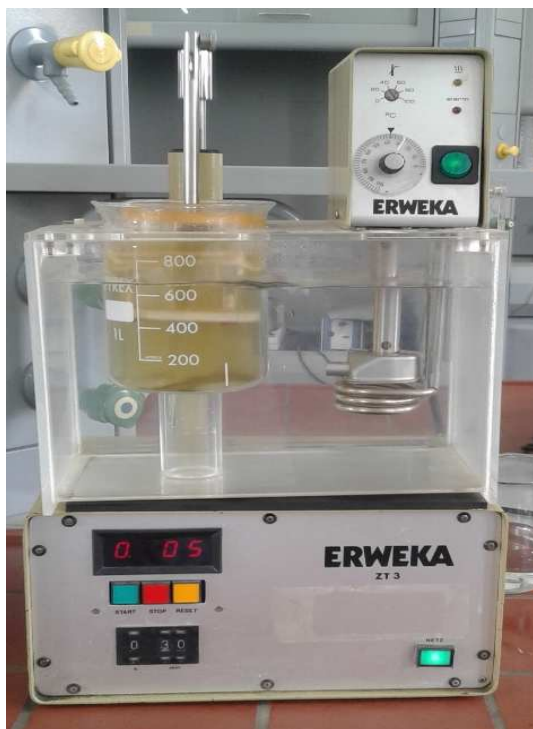
Plate 5: Disintegration testing machine
