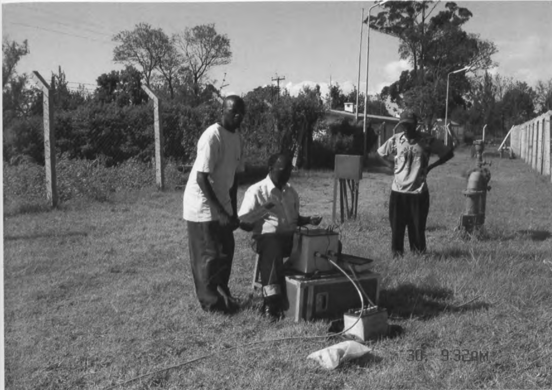
Figure 4.2 Field data collection using SYSCAL R1 switch 72 ERT meter.
