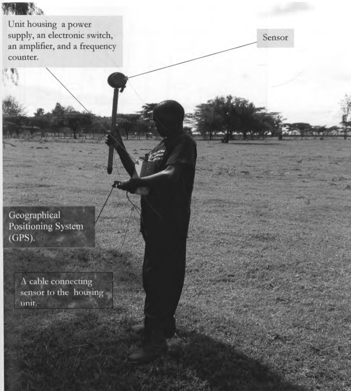
Figure 4.3. SINTREX Total Field Proton Precession Magnetometer used in the field.
