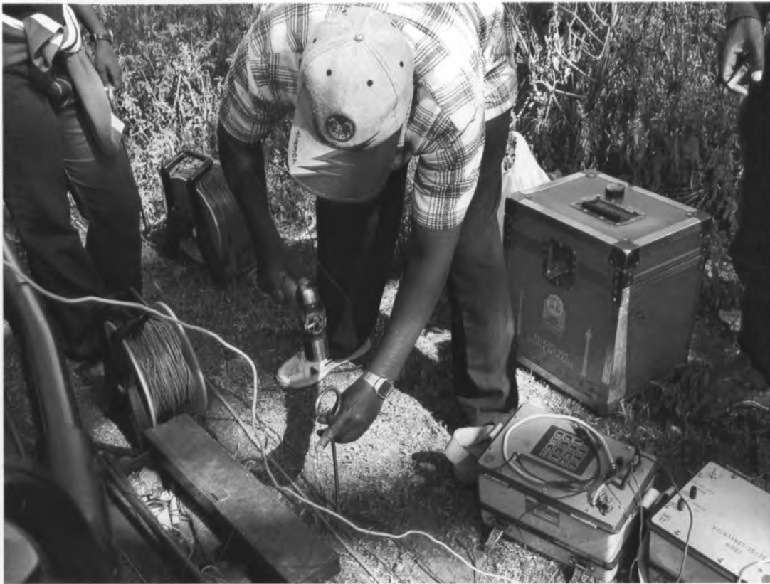
Figure 4.1 SYSCAL R2 electrical resistivity equipment which was employed in data collection.
