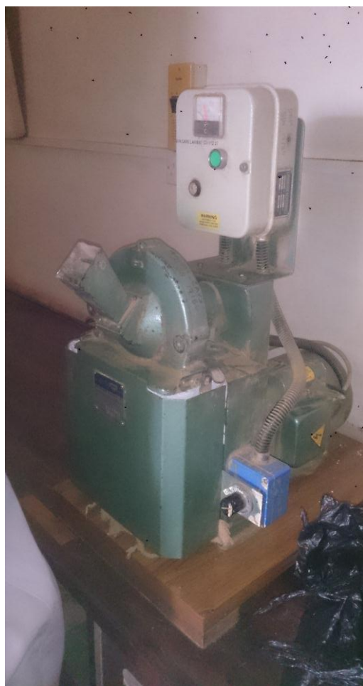
Figure 8: Grinding machine used to grind three dry plant materials
