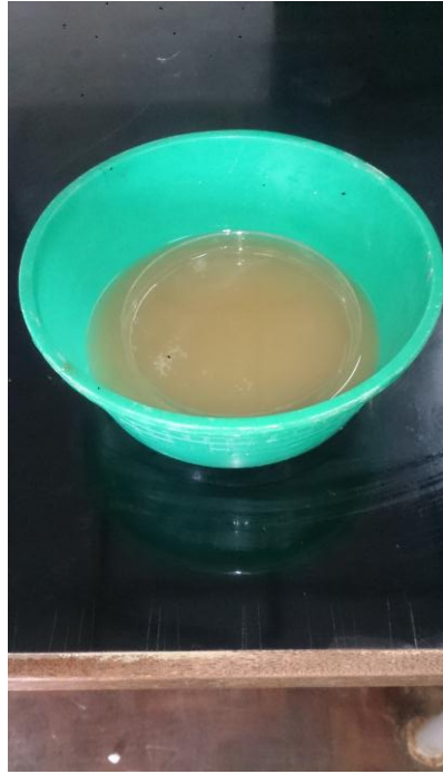
Figure 15: A plastic petri dish floating on a mixture of concentrated salt solution and fecal material
