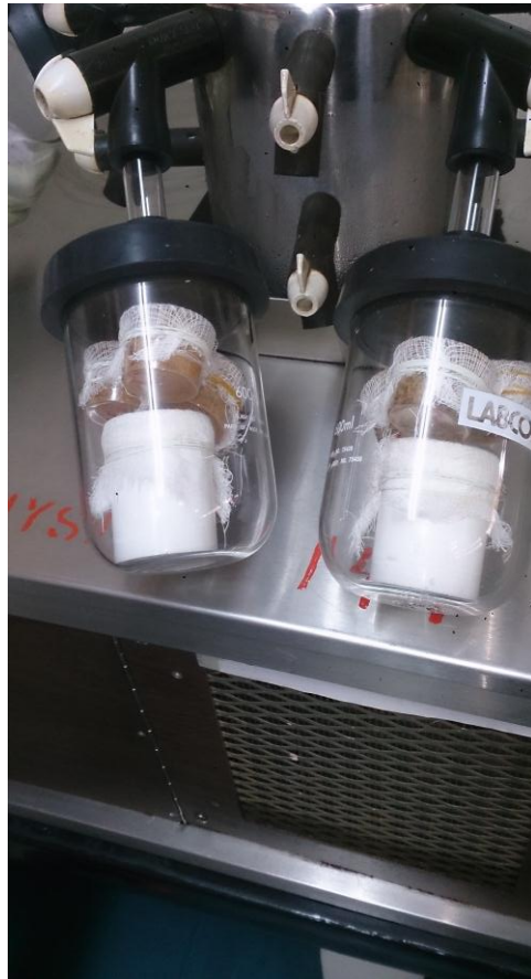
Figure 11: Aqueous extract of Allium cepa mounted on a freeze drier
