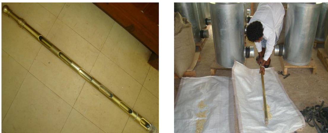
**Plate 4.10** Compartmentalized double tube sampling spear for sampling grain in the containers.
