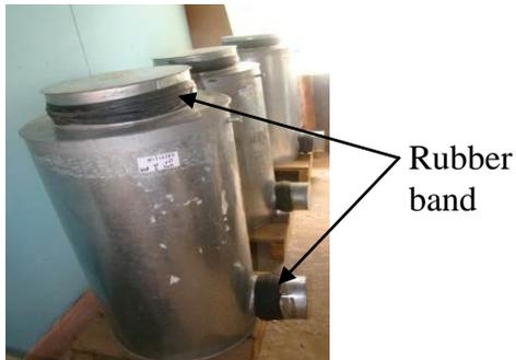
**Plate 4. 5** 100-kg metal silo with the in-let and out-let sealed with rubber band (T1)
