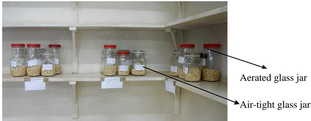
**Plate 4.4** Aerated and air-tight glass jars with maize at ambient conditions in the laboratory.
