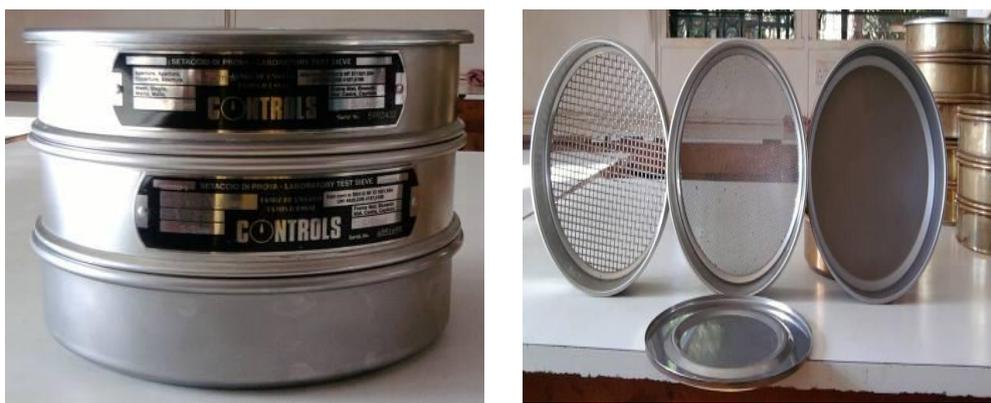
**Plate 4. 9** Sieves (Endecotts Limited, UK) of 4.7mm and 1.0mm used to separate grains, insects and dust.
