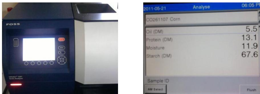
**Plate 4.13** Infratec™ 1241 Grain Analyzer showing some readings on protein, oil, starch and moisture content (left)
