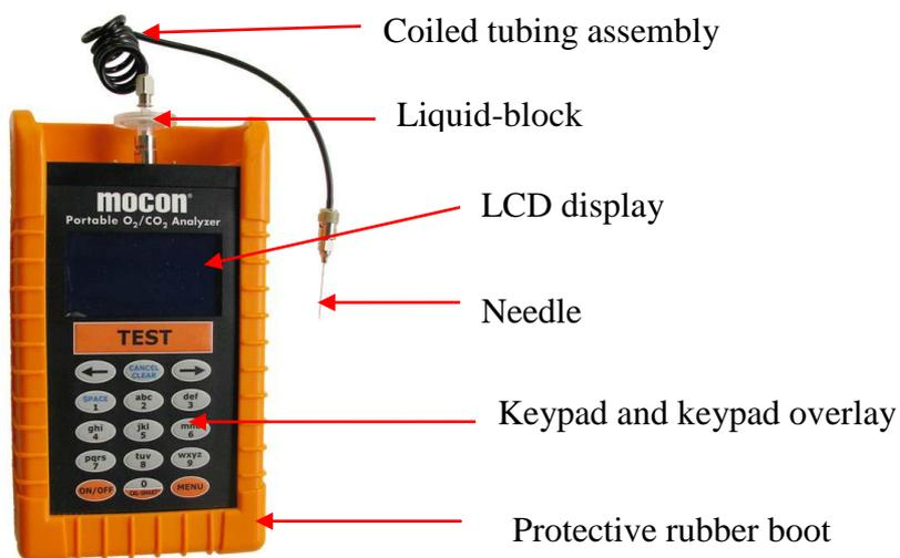
**Plate 4. 12** Mocon PAC CHECK<sup>®</sup> Model 325 used to measure oxygen and carbon dioxide levels
