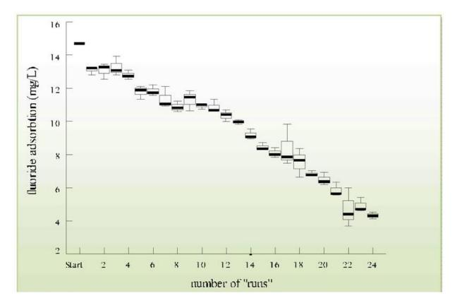
Figure 4.4: Box plot showing the gradual reduction of fluoride binding effect in a Laterite filter after repeated exposure to divisions of 14.7 Mg/L NaF solutions.
